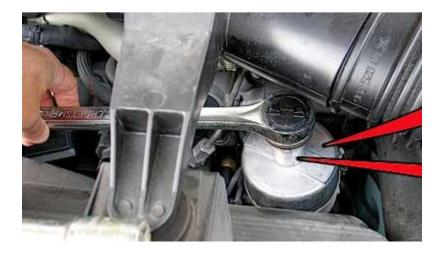
Remove the filter top using a filter removal cap and a 22mm wrench as shown with the arrows.
