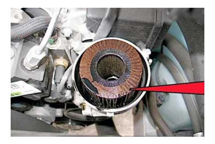
Remove the filter and replace with the new. Add oil until about 3/4 full.
