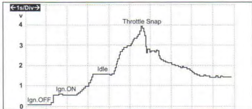
Figure 217 Rail Pressure Sensor Signal
