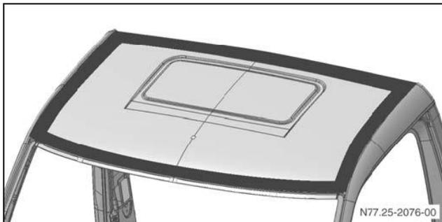
**Adhesive for fitting wind deflectors should be applied in the area shown**
