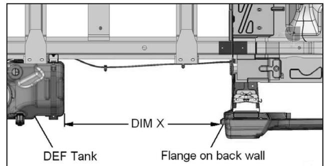
Top view DEF tank location (Chassis Cab)
