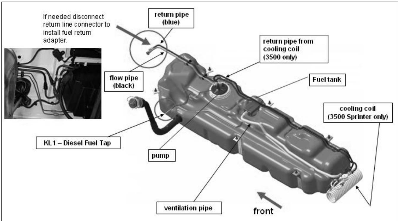
Diesel Fuel System 26.4 gal / 100 L
