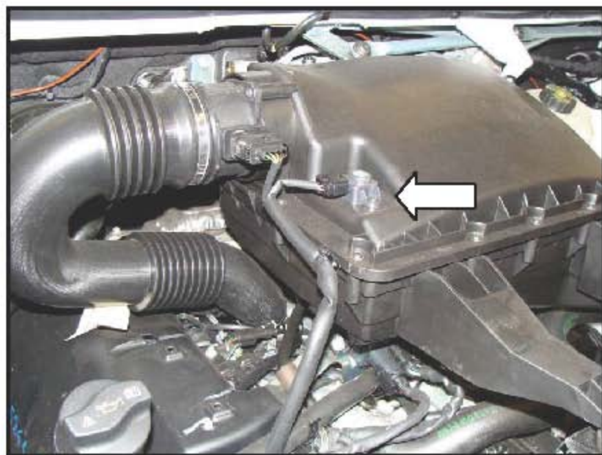
B28/19 - Pressure sensor downstream of air filter
