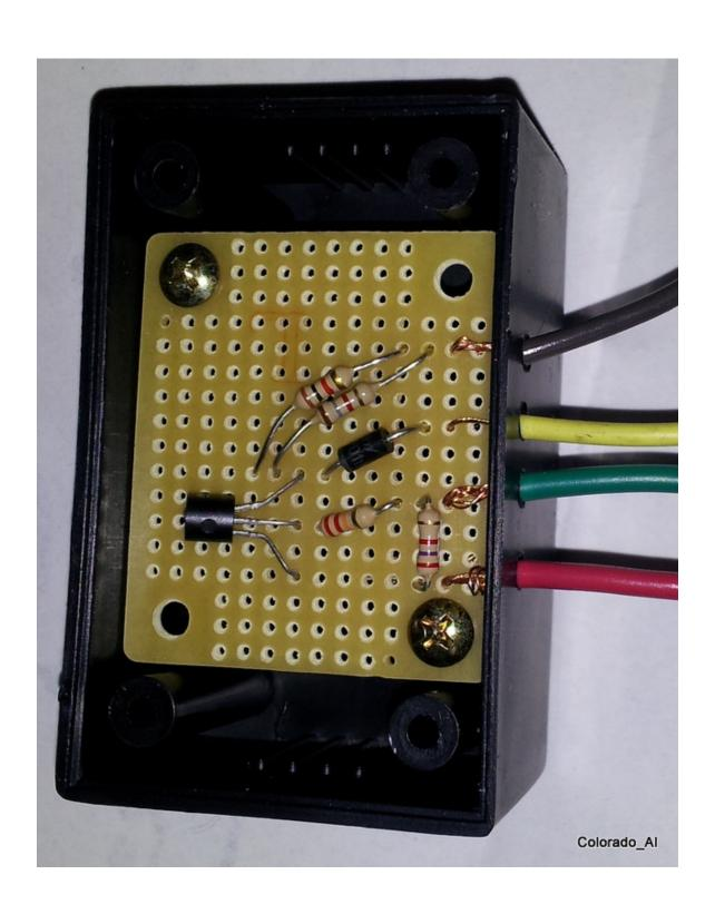
So, after building the circuit, I connected it to the ECU, and unplugged the EGR cable at the EGR. All 4 wires are piggybacked to wires at the ECU, connected with wire taps.
