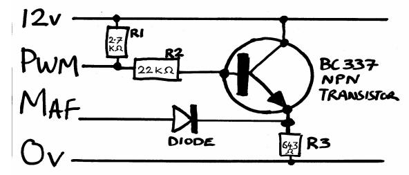
PWM is the pulse modulated signal wire for the EGR MAF is the signal wire from the MAF
