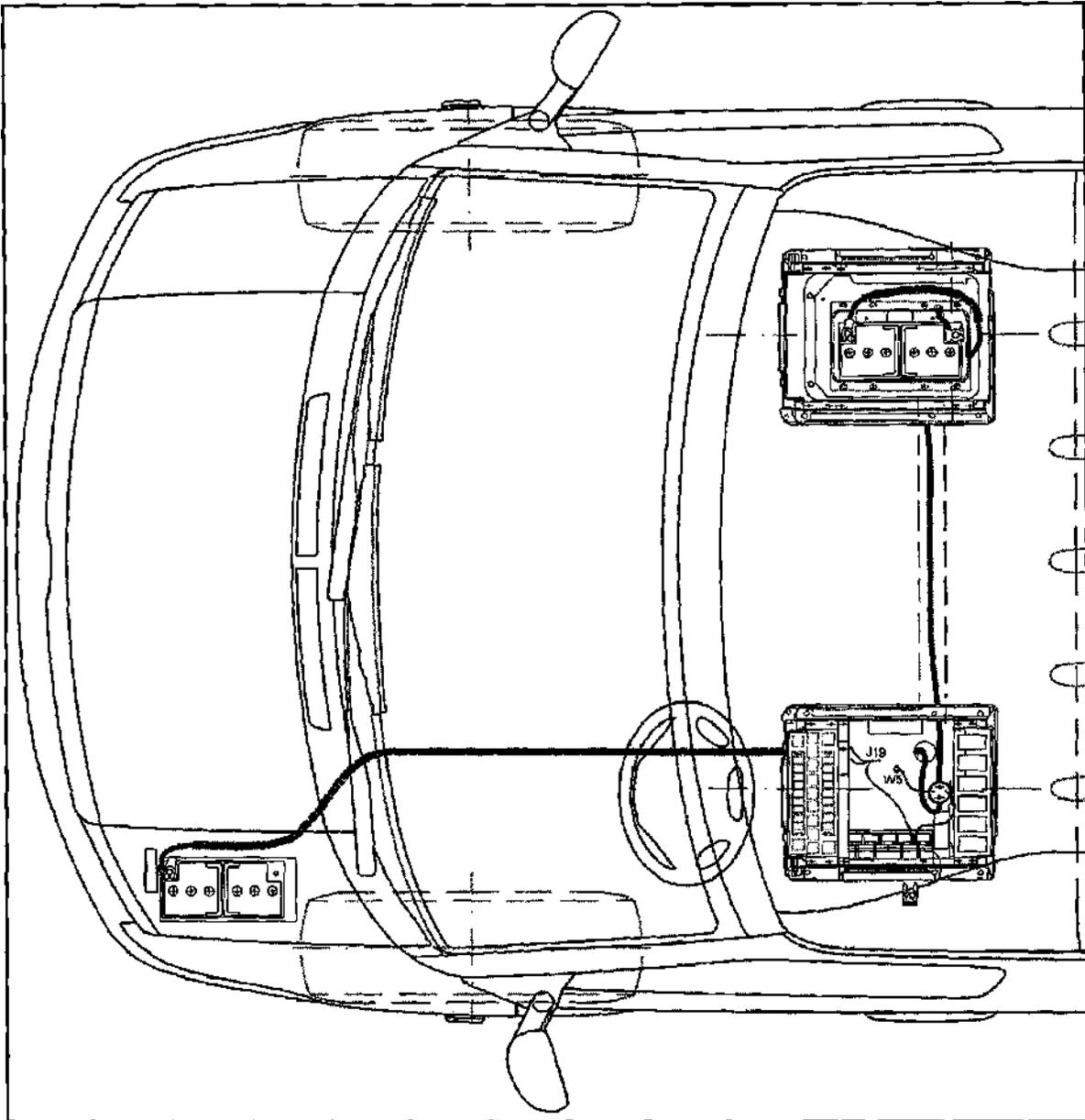
Fig 10, Auxiliary battery wiring layout
