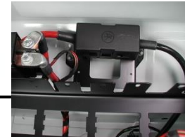
Install an electrical connector for all aftermarket components after cut-off relay
