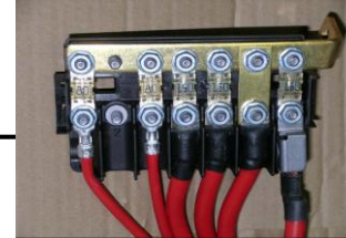
Pre-Fuse Box located on battery (+) pole
