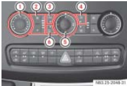
Control panel for the air-conditioning system
